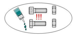
Glue all screws, nuts and sleeves with loctite. (Not less than 5 Drops!)
