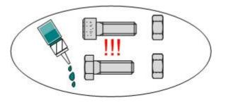
Glue all screws, nuts and sleeves with loctite. (not less than 5 drops !)(except for lock nuts)
