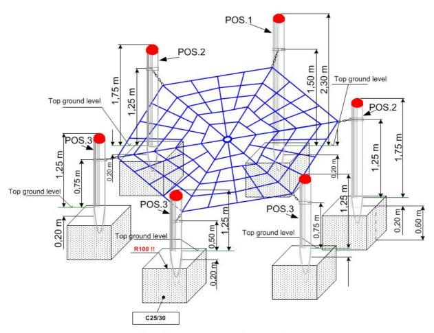
Round off all foundation edges (min.R = 100 mm)! Sizes of fundations are "4-5" (natural ground).
