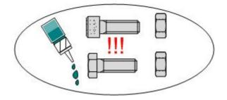
glue all screws, nuts and sleeves with loctite. (not less than 5 drops !) (except for lock nuts)
