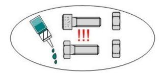
Glue all screws, nuts and sleeves with loctite. (not less than 5 drops!)(except for Nyloc nuts)
