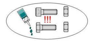
Glue all screws, nuts and sleeves with loctite. (No less than 5 drops!) (except for Nylock nuts)
