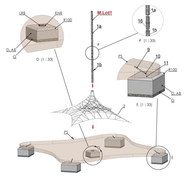
Place Pos.2 with marked side ("Top side") over Pos.20 and then install Pos.1A, Pos.1B and Pos.16.
