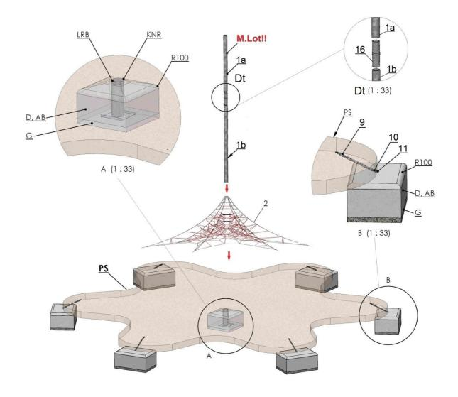
Place Pos.2 with marked side ("Top side") over Pos.20 and then install Pos.1A, Pos.1B and Pos.16.
