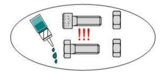
Glue all screws, nuts and sleeves with loctite. (not less than 5 drops!)(except for Nyloc nuts)
