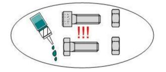
glue all screws, nuts and sleeves with loctite. (not less than 5 drops !) (except for lock nuts)
