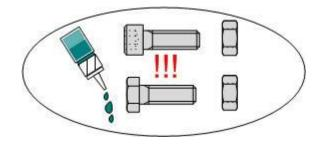
Glue all screws, nuts and sleeves with loctite.
