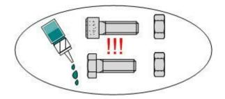
Glue all screws, nuts and sleeves with Loctite. (not less than 5 drops !) (except for Nylock nuts)
