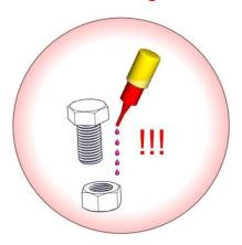
glue all screws, nuts and sleeves with loctite (not less than 5 drops !)
