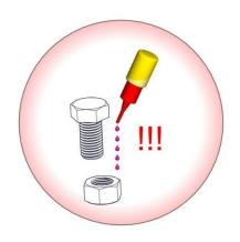
glue all screws, nuts and sleeves with loctite. (not less than 5 drops !) (except for lock nuts)
