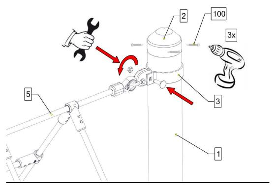
Fixed anchor/plug fastening for M12-15-30/110
