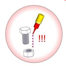
All screws, nuts and bushes have to be secured with Loctite
