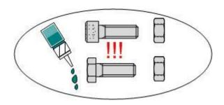
Glue all screws, nuts and sleeves with loctite.
